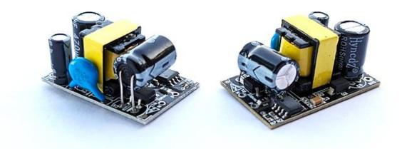
This power supply module can be used to power from DIY to any industrial projects that need isolated AC to DC conversion. The module is capable of supplying full load current constantly for longer period. Thus, making it perfect choice for all types of loads.
